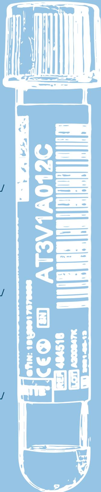
Standardized label and barcode placement according to ISO guideline Code-128 for optimal readability on all common laboratory equipment
