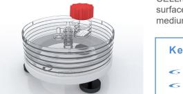
CELLring assures an exact horizontal position of CELLdisc™ compensating surface irregularities, e.g. of a working bench or an incubator. Thus, cells and medium distribute evenly in every single layer of your CELLdisc™.
