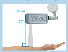
Correct focus position is indicated by the text in the image being clearly legible:
