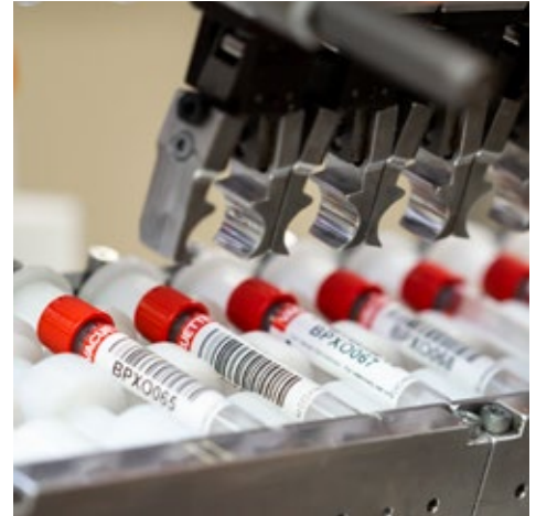
VACUETTE® barcode tubes are labelled during the manufacturing process.
